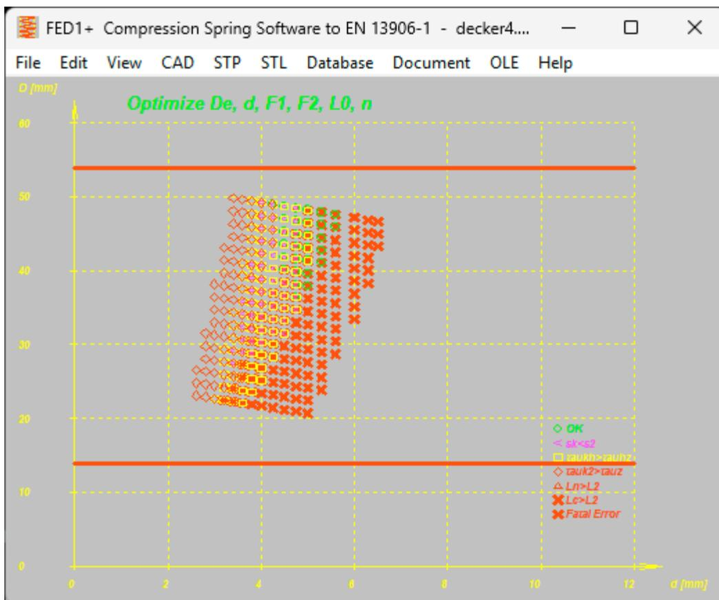
The labeling of the vertical axis with the coil diameter has been changed from "De" to "D." The upper limit is "De max," and the lower limit is "Di min." For the calculated springs, the wire diameter is marked "d" and the mean coil diameter is marked "Dm" (not "De").
